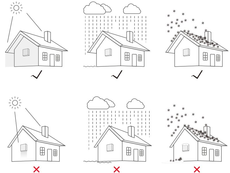
▲ Figure4.1 Recommended Installation locations
